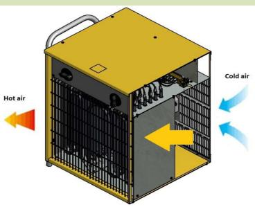
The device works on the principle offorced convection . The air flow is forced fan. Cold air is drawn in the back of the unit. Further washes flowing from the heater receives heat. The heated air is expelled in front of the heater. The device has a thermostat for the regulation temmperatury 5-35 °C. The unit area equipped with thermal protection is acting automatically. The unit features: ventilation, heating with half the power, heating at full power. Device has cooling thermostat.
