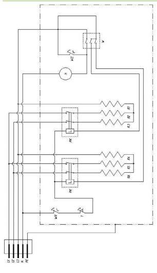
Phase L1 Ν Neutral WR Thermal cut-out **Ambient thermostat** WZ R1 **Heating element** R2 **Heating element** R3 **Heating element** R4 **Heating element** R5 **Heating element** R6 **Heating element** Т **Thermostat** Motor M PK Relay
